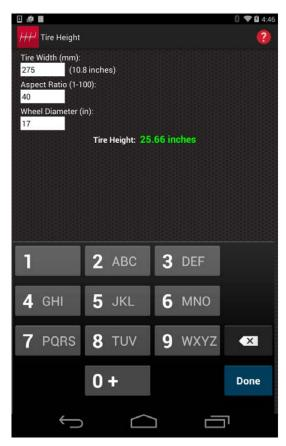
The TREMEC Tire Size Calculator will calculate the tire height and width on a metric size tire for you and convert it to the easier to understand good old American inches.
