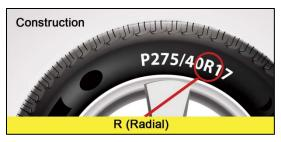
**Construction.** The letter "R" in a tire size stands for Radial, which means the layers run radially across the tire.
