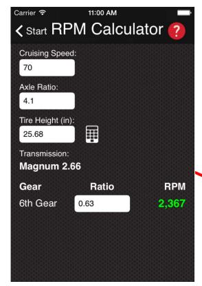
This calculator is designed to give the approximate engine RPM (revolutions per minute) based on data entered.
